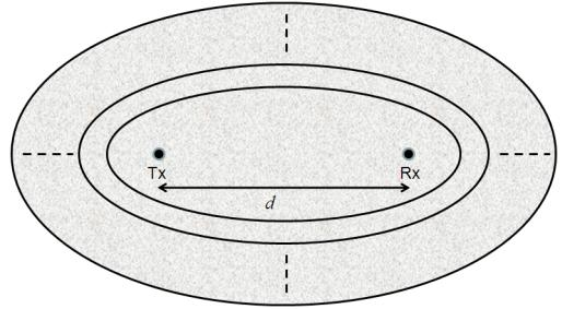
Fig. 1. Geometrical model for indoor UWB communication.
